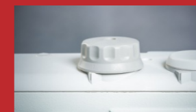
压脚交互量旋钮（交互量可调）最大交互量可达9mm，安全爬坡不同厚度的缝料层 Alternating press feet stroke adjustment dial (alternating feet stroke height can be adjusted) the maximum stroke can reach 9mm, safely climbing over different thickness of sewing material
