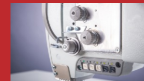
多功能机头按键（智能操作）如自动剪线，自动倒回针，气动抬压脚/压脚交互快速调节机构 Multifunctional machine head buttons (intelligent operation) such as automatic thread trimming, automatic back-latching, pneumatic presser foot lift/alternative presser feet quick stroke adjustment mechanism
