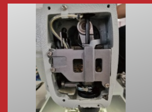
针杆无油方式实现清洁缝制 Adopted Non-oil lubricated needle bar parts for clean sewing
