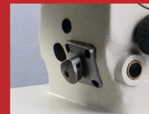
一步两点，三步四点可切换 Switch for 1 step 2 points, 3 step 4 points
