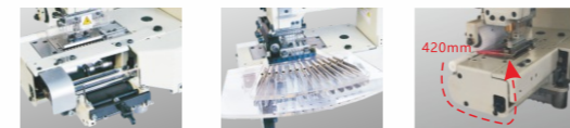
PMD 松紧带装置 Elastic Device PTV 打褶装置 Shirring Device 筒型周长420mm Cylinder circumference 420mm
