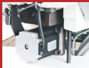
步进电机送料系统(仅限于SR) Stepping motor feeding system (Available in SR)
