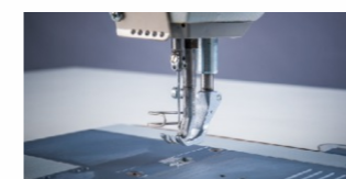
压脚抬高高度最多可达20mm The presser foot lift can be raised up to 20mm
