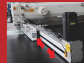
X向无限缝制 Infinite sewing in the direction of X-axis
