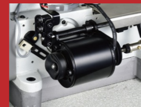
剪线电磁铁 Electric trimmer device
