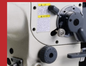
缝纫摆幅调节 Sewing width dial
