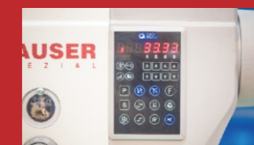
一体化电控（直驱电机） Integrated electronic control (direct drive motor)
